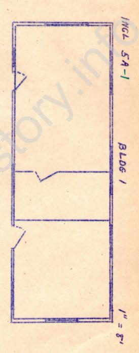
Wood frame structure, 2" X 6" floor joists, 1" X4" pine flooring over 7/8" pine sub floor, 2" X \$2 studding end rafters. Composition roll roofing on pine sheathing. Wells inside end out of gypsum board, Ceiling end partitions of gypsum board. .
