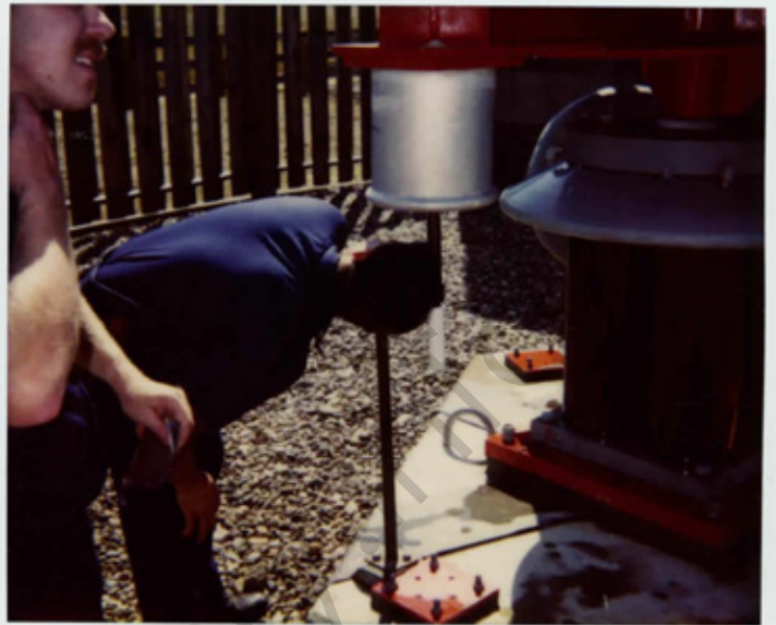
MK1 Brazier inspecting tower ball gaps
